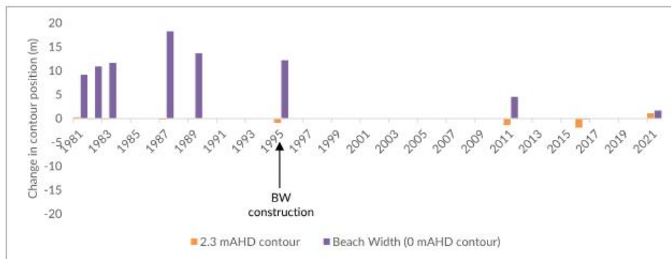
Figure 11: Northern beach (north of access road) shoreline position relative to 1981 (profile 56008)
