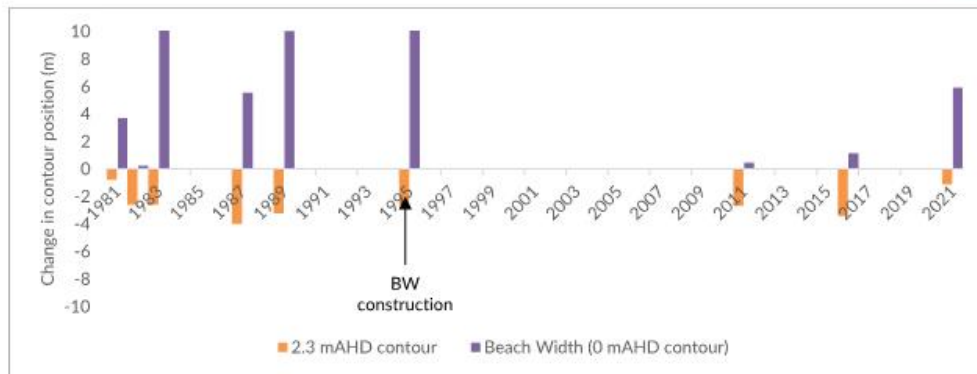
Figure 10: Northern beach (wave shadow) shoreline position relative to 1981 (profile 56009)
