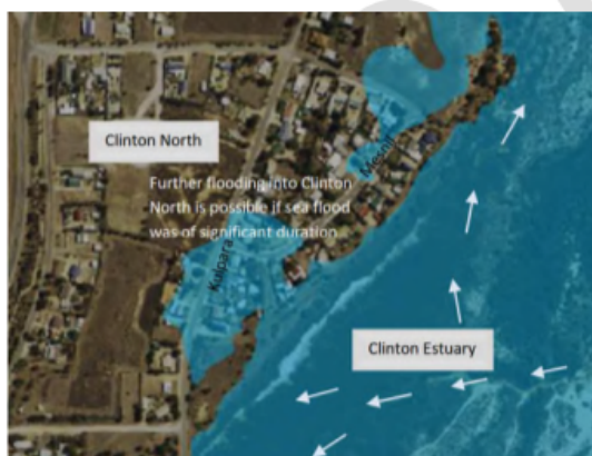
Figure 1 – Flood extent at +3.1 mAHD (from Stage 1: State of Play report)
