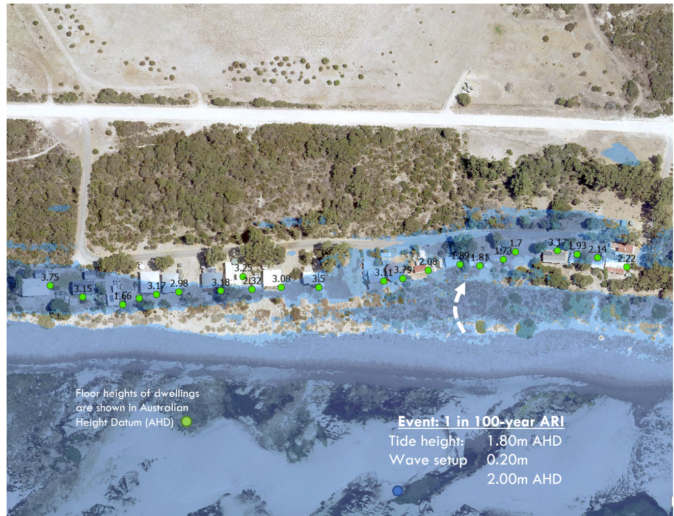
Figure a. Storm modelling for the event 1 in 100-year ARI storm surge event for current risk. Wave runup has not been included so as to evaluate the likelihood that this event would penetrate through the dune system. Depending on the duration of the flood event, sea-flooding may penetrate through the dunes and cause inland flooding.
