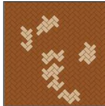
Brick Paving (Herringbone)
