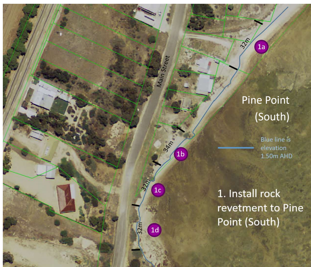
Figure 2:3 Proposed rock revetment sections for Pine Point (south).
